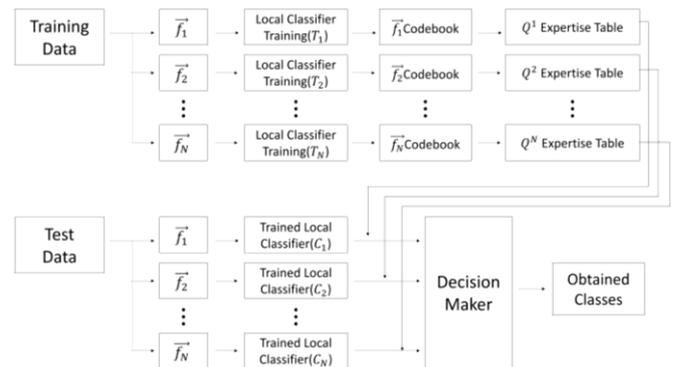
Fig. 3. Multiple feature-based classifier model [7].
