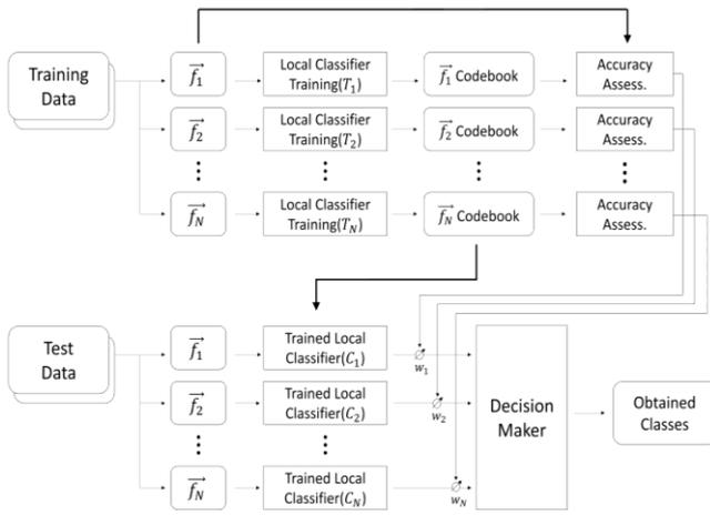
Fig. 2. Partitioned feature-based classifier model [6].
