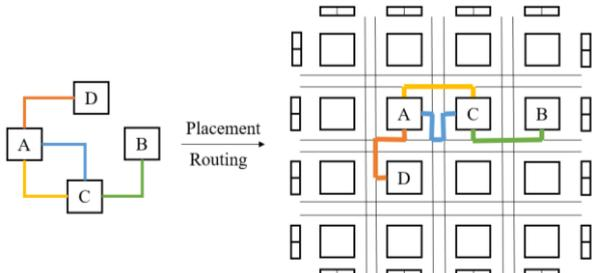
Fig. 2. Example of placement and routing results on island style FPGA.
