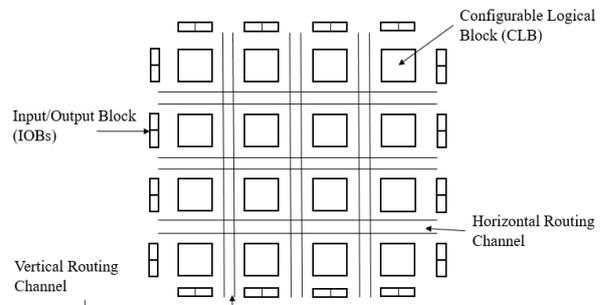
Fig. 1. General architecture of island style FPGA.
