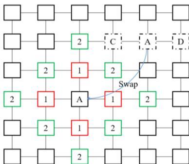
Fig. 7. Example of swap operation and distance between CLBs.
