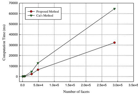
Fig. 6. The computation time according to the number of facets.
