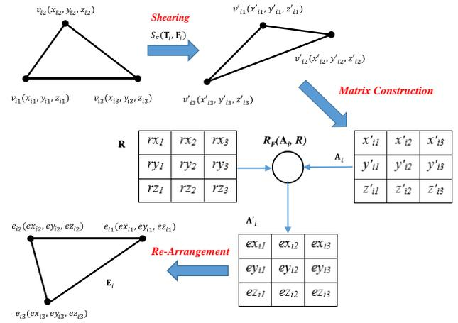
Fig. 3. The random encryption process used for each facet.
