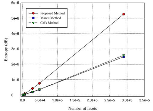
Fig. 5. The entropy of the proposed method according to the number of facets.
