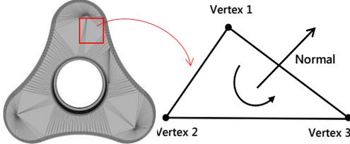
Fig. 1. The structure of 3D triangle mesh.
