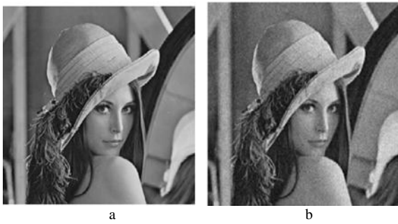
Fig. 1. (a) Lena test image. (b) Lena Test Image corrupted with Gaussian noise of Zero mean with standard deviation of 50.
