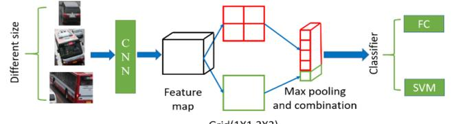
Fig. 7. Principle of SPP.
