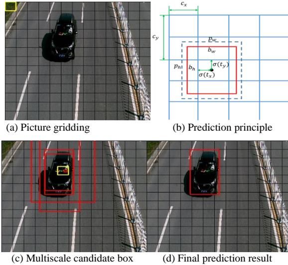
Fig. 1. Yolov2-tiny detection procedure.
