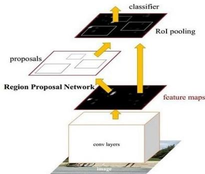
Fig. 3. Faster R-CNN architecture [45].
