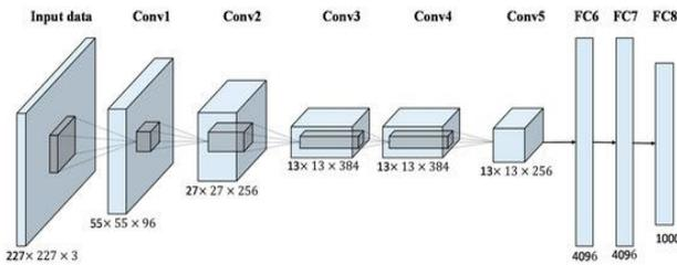
Fig. 1. AlexNet architecture [47].
