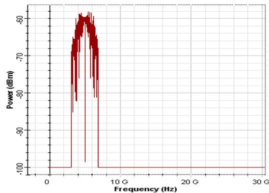
Fig. 12. RF spectrum regenerated at the 5GHz working frequency
