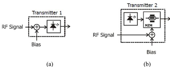
Fig. 1. IM-DD technique (a) Directly modulated RF (b) Using external modulator
