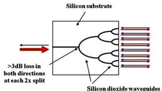
Fig. 3. A planar lightwave circuit (PLC) splitter
