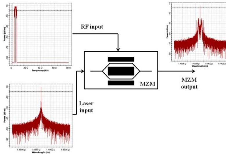
Fig. 6. Modulation of a Mach Zehnder modulator at the CS
