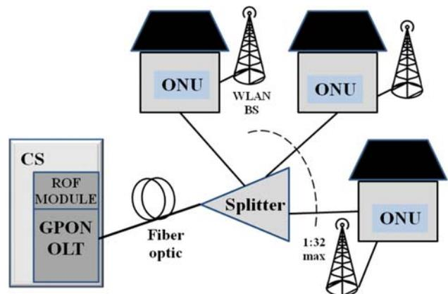
Fig. 2. A typical RoF on GPON architecture
