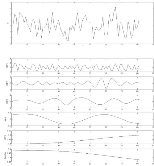
Fig. 8. Input signal  $x(t)$  (top). Set of IMF's  $x(t)$  (bottom).
