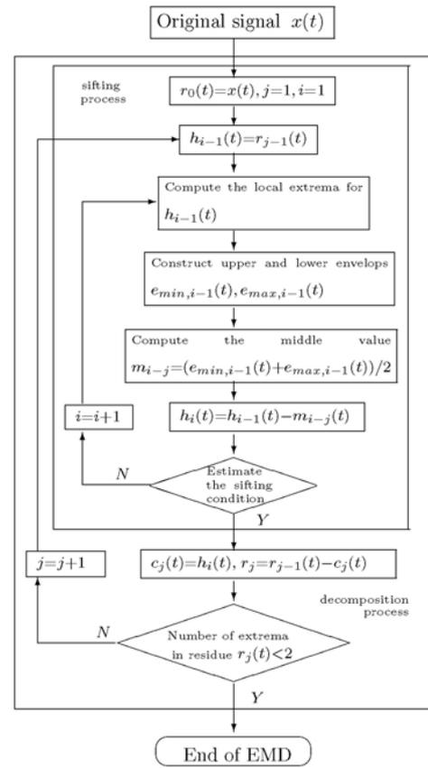
Fig. 7. The algorithm of the empirical mode decomposition.
