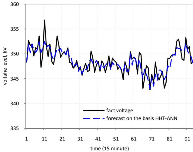
Fig. 16. Forecast of voltage magnitude (node 13) for a lead time interval of 15 minutes.
