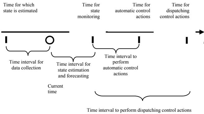
Fig. 1. Time diagram of events in the system for monitoring, forecasting and control in EPS.
