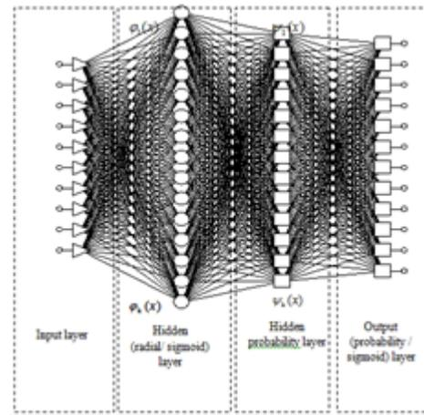
Fig. 4. The generalized multi-layer perceptron structure.
