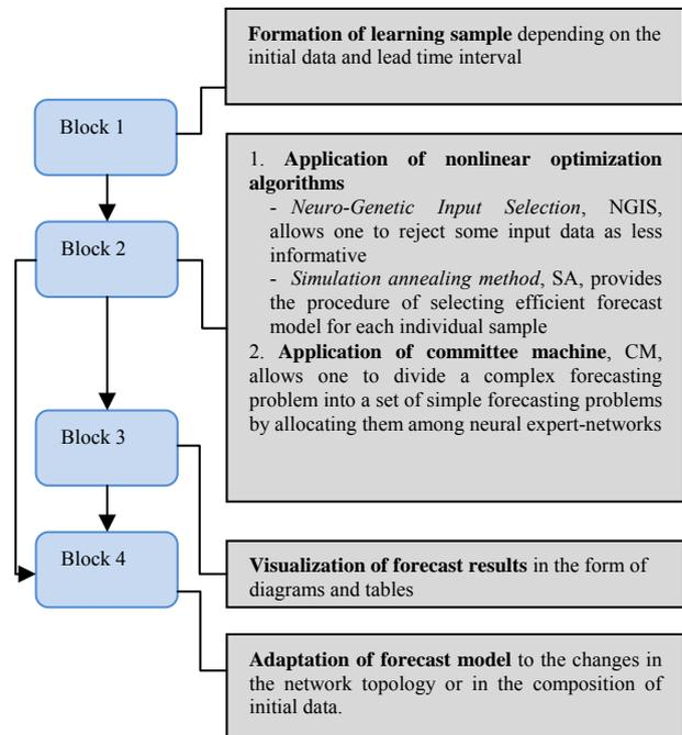
Fig.5. Forecast subsystem of the ANAPRO software.
