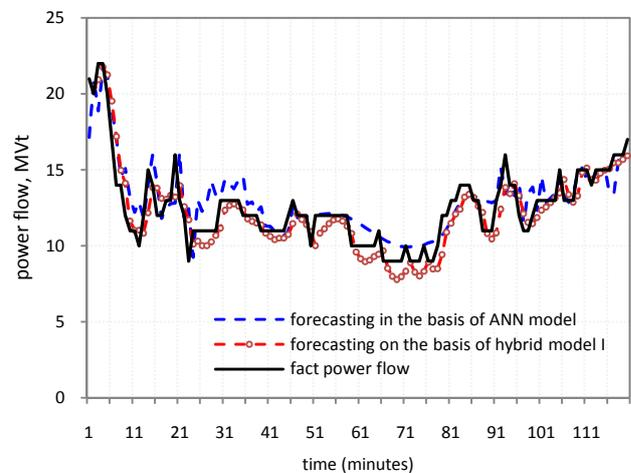
Fig. 15. Forecast of active power flow for a lead time interval of 1 minute.
