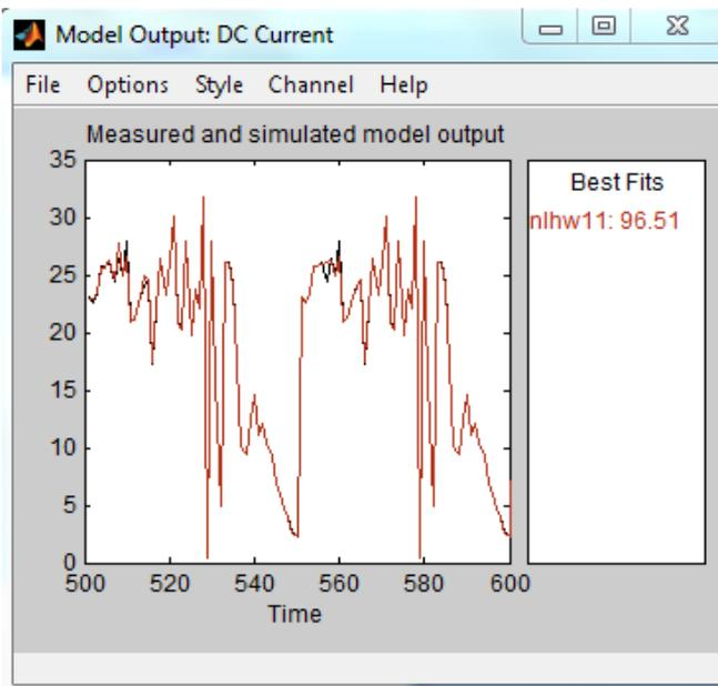
Fig. 4. Original output (Black) and estimated output (Brown) for the same input signal
