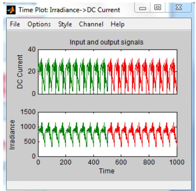
Fig. 3. Input and output data measured for PV system under normal operating
