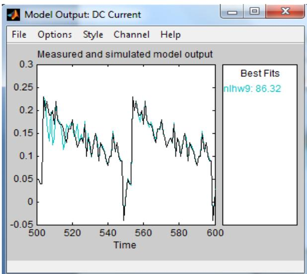
Fig. 8. Original output (Black) and estimated output (Light Blue) for the same input signal
