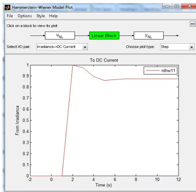
Fig. 5. Linear transfer function of Step Plot type
