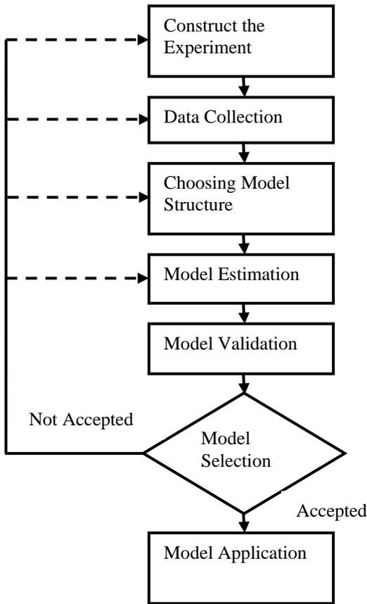
Fig. 1. Process of System Identification using HW method
