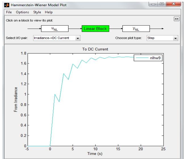
Fig. 9. Linear transfer function of Step Plot type
