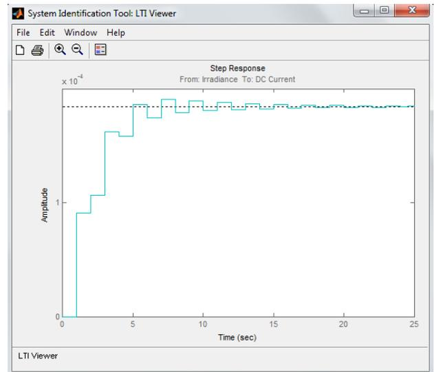
Fig. 10. Step Response for shading operation
